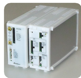
300W (ファンレス) 幅:43mm,奥行:207mm,高さ:132mm
